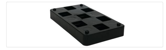
The K-Block 45 series is designed to accurately fit the width of rafters and other planed 2" wood, but is also used for distance adjustment and leveling of medium-heavy tasks such as doors and windows. The countersunk screw holes provide secure mounting.
